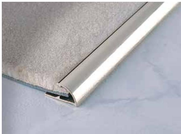
CARPETEC trim profiles compress to hold flexible flooring, such as natural fiber carpeting. By pressing the profiles, they close slightly to clamp the flooring, hiding and protecting edge imperfections.
